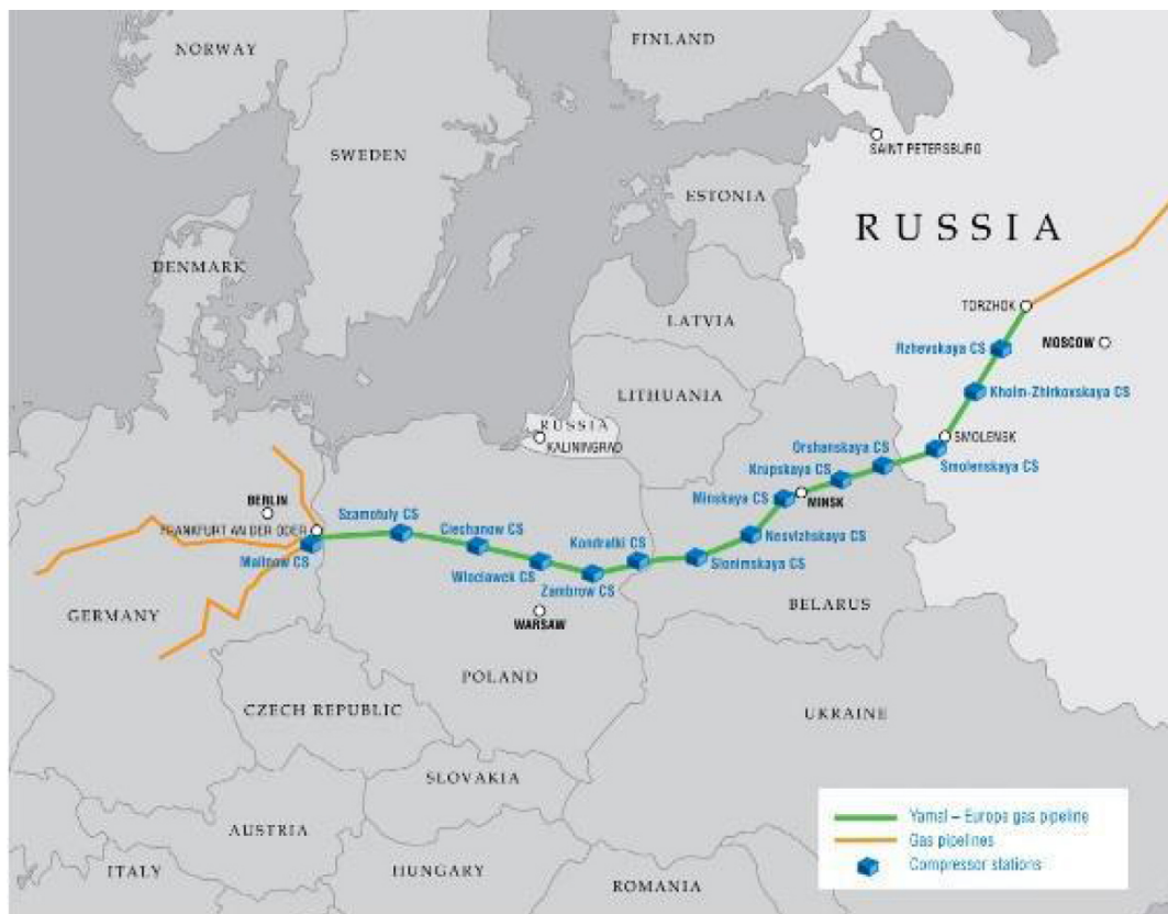
Figure 3-3 Yamal Europe gas pipeline
